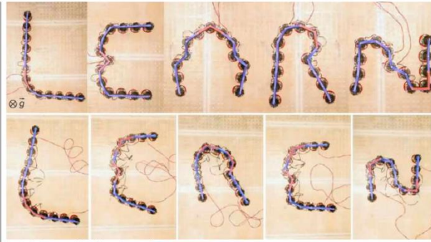
Top: A robotic metamaterial spells the word 'LEARN'. A metamaterial is a special material whose properties are not determined by its chemical composition alone but also by its structure, giving rise to unusual properties. COULAS LAB/UNIVERSITY OF AMSTERDAM
